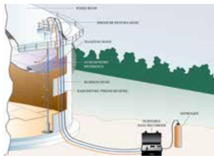
The pressure head at the base of the tank is transferred to the transmitter using a nitrogen bubbler system.
